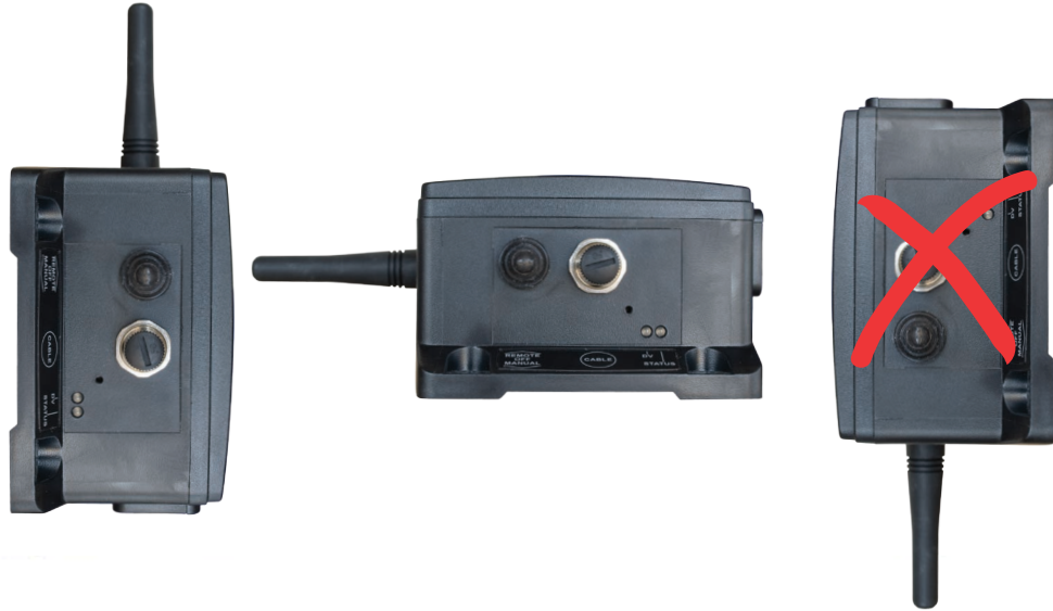
Figure 5.2 How to mount the Central Unit.
