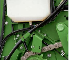
the chain oil is applied at just the proper rate.
