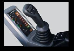
installed on the right hand joystick reduces fuel consumption when the excavator is temporarily idled.
