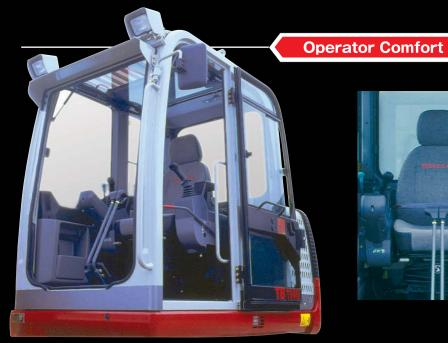
minimises noise levels and vibration within the operators station for added operator comfort and awareness of the excavator's operating and worksite condition.
