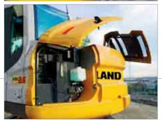
iesel tank with level indicator. Electric fuel pump and windscreen washer reservoir.
