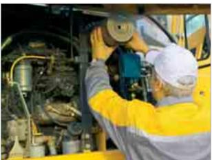
uel and air filters check. Oil filter in vertical position.
